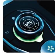
Vehicles converted with Sequent gaseous injection systems are equipped with a push-button changeover switch with acoustic indicator (Buzzer), on which a gas level indicator consisting of 4 green LEDs is integrated.
