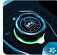
Vehicles converted with Sequent gaseous injection systems are equipped with a push-button changeover switch with acoustic indicator (Buzzer), on which a gas level indicator consisting of 4 green LEDs is integrated. This is a one-position switch and is called “One-Touch”. Fuel change (gas or petrol)
