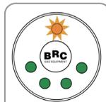
**EMPTY TANK:** ORANGE CENTRAL LED FLASHING AND CONTINUOUS BEEP
